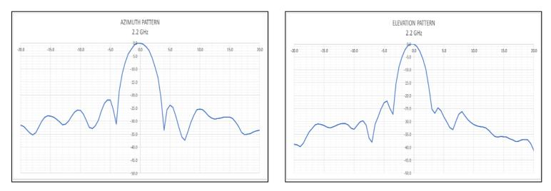
S-Band patterns taken using the M2 Antenna Systems FGFD-2-SC-XC-1 Dual-Band Feed, installed on a 3.7M Reflector at 2.2 GHz.
